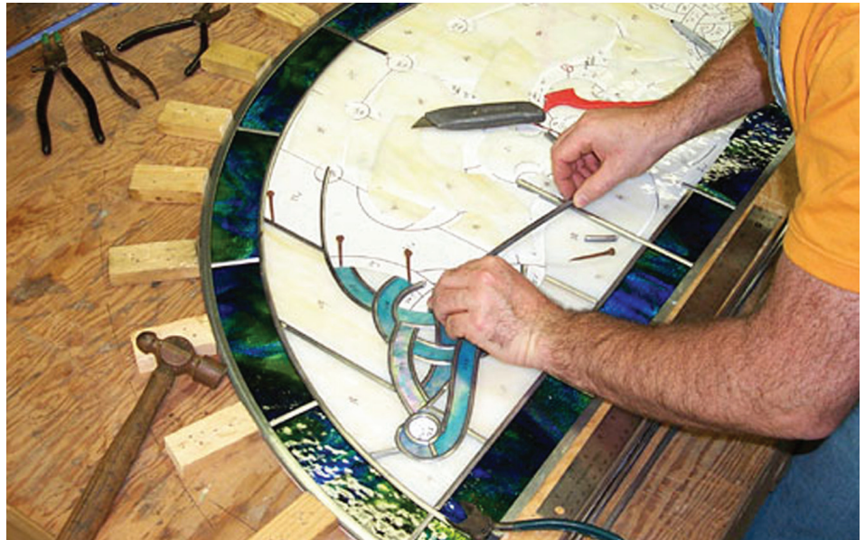
Once the glass pieces have been cut according to the design, they are fitted into the channels of lead came and laid out on the master pattern.
